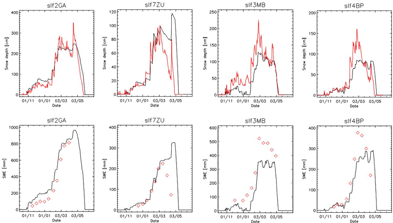
Figure 6: Observed (red) and simulated (black) snow depth (above) and snow water equivalent (below) at four selected stations in different regions. The stations and regions (as calibration centres) can be seen in Figure 7.
