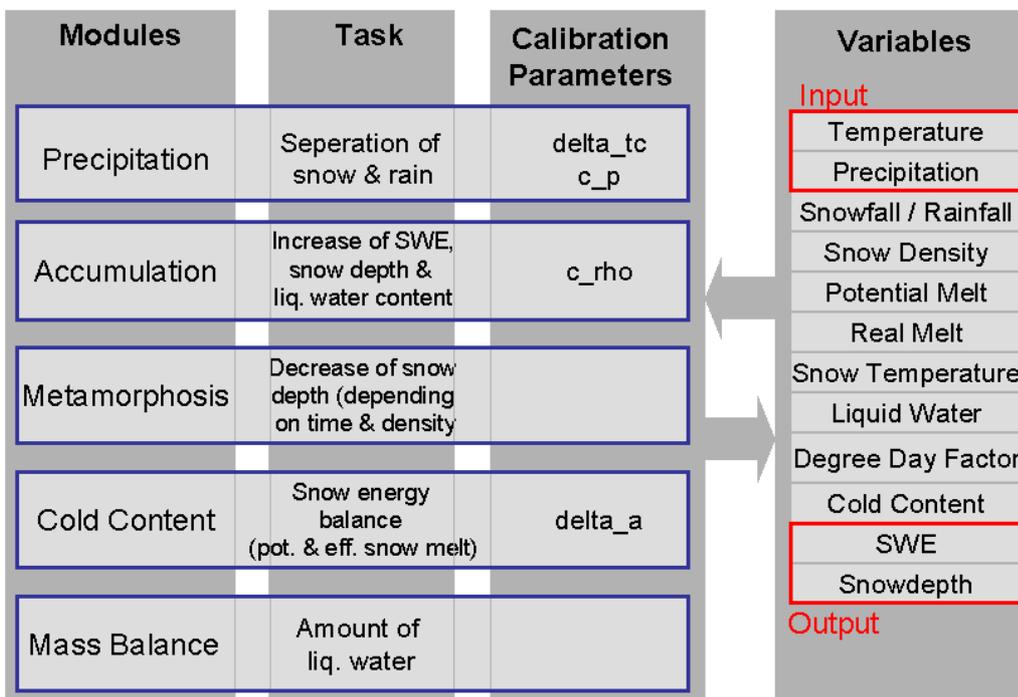
Figure 1: The five modules of the snow model that are responsible for the calculation of the snow pack and their tasks. The four calibration parameters can be used for calibrating the model. The variables are interchanged between the modules.
