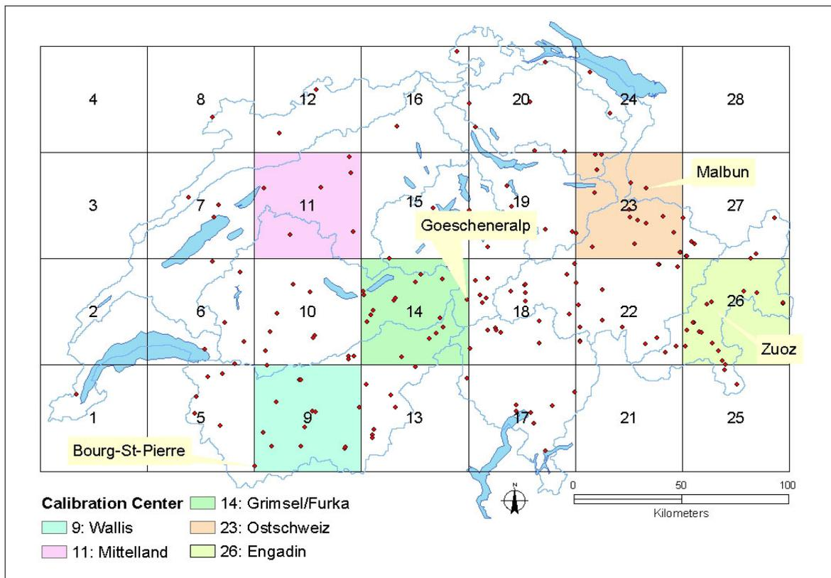
Figure 7: Calibration centres as referenced in Table 2 (numbered boxes filled with colours) and all the snow gauges relevant for this study (red points). The four stations discussed in this work are labelled.
