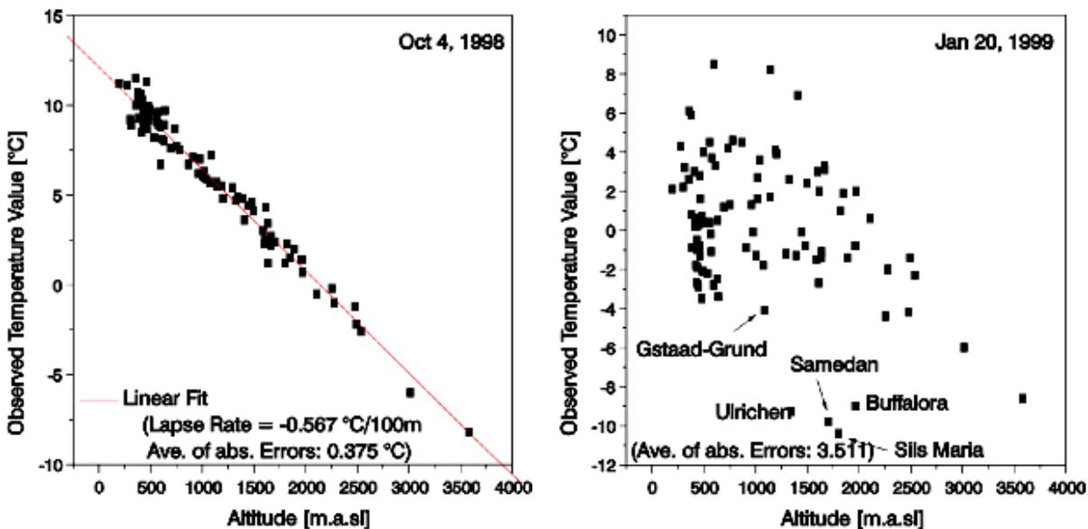
Figure 5: Temperature-elevation relationship for Oct 4, 1998 (left) with minimal interpolation error and for Jan 20, 1999 with a high interpolation error due to inversion layers
