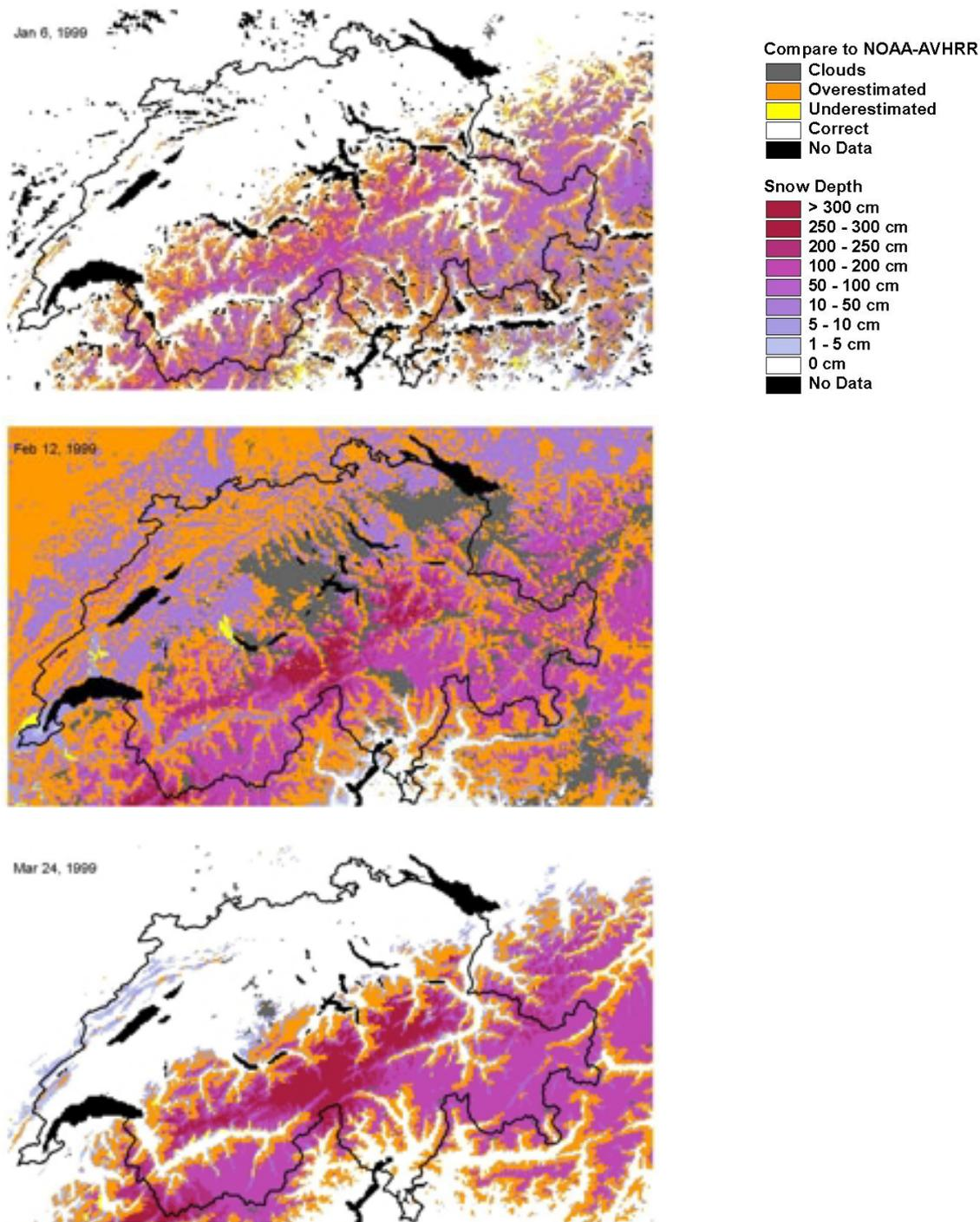
Figure 8: Comparison of simulated snow maps with snow maps derived from NOAA/AVHRR data on Jan 6 (top), Feb 12 (middle) and March 24, 1999 (bottom). Orange: overestimation by the snow model, yellow: underestimation by the snow model. Light blue to dark red: snow depth from 0 cm to > 3 m. Gray: Clouds, Black: no data and lakes.
